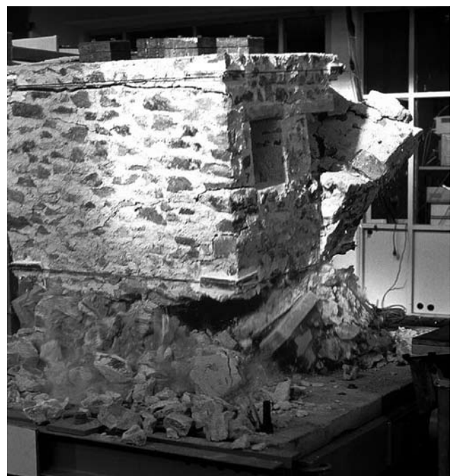
Fig. 8a and 8b Results of a shaking table test using a model of a rural stone house with wooden floors; (a) without steel ties, (b) with steel ties
