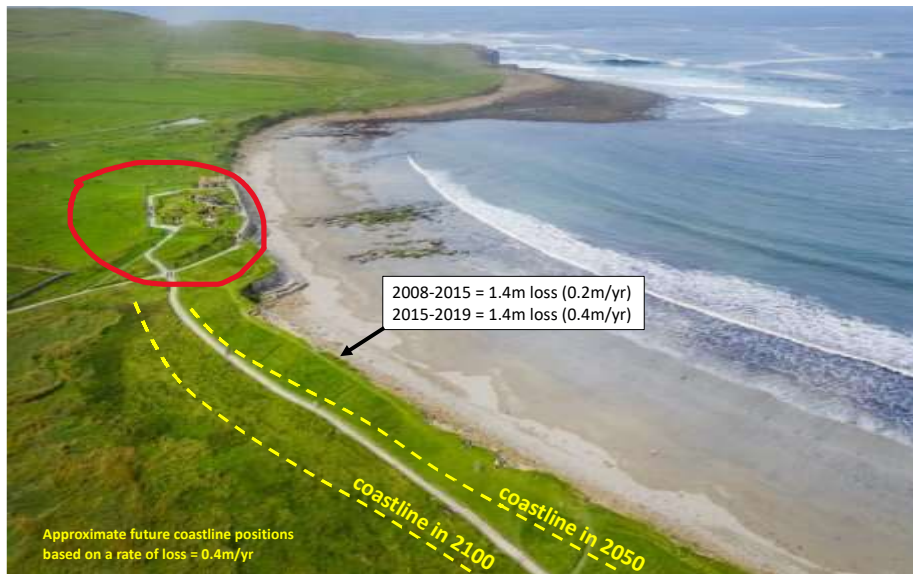
Figure 9. Illustration of potential coastal retreat at Skara Brae based on annual loss of 0.4 metres (Data source: Dynamic Coast )
