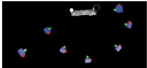
Fig. 4. Camera stations to produce a 3D Model for the left Gate of the stage of Jerash Southern Theatre
