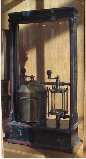
Fire pump, Savery system 1698, 18th century reconstitution (Photo: Wikimedia Commons)
